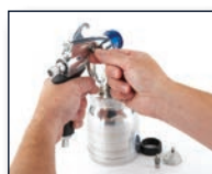
2 Slide trigger lever to release needle
